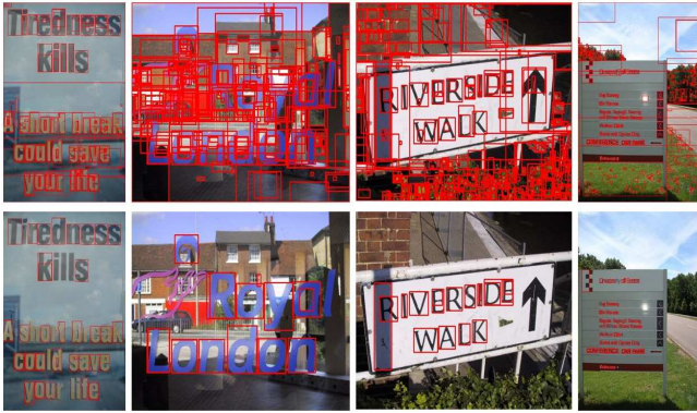
Fig. 3. Top row and bottom row: character candidates before and after character classification.
